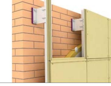
Fiber cement is a composite building material composed of cement, quartz sand, cellulose fibers and water. The cellulose fibers in the composition act as a reinforcing agent, that is, they give the required strength to the material.
