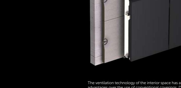
The ventilation technology of the interior space has a number of advantages over the use of conventional coverings. Due to this, a constant dry microclimate is maintained, the danger of dampness of the building walls and the heat-insulating layer is prevented.
